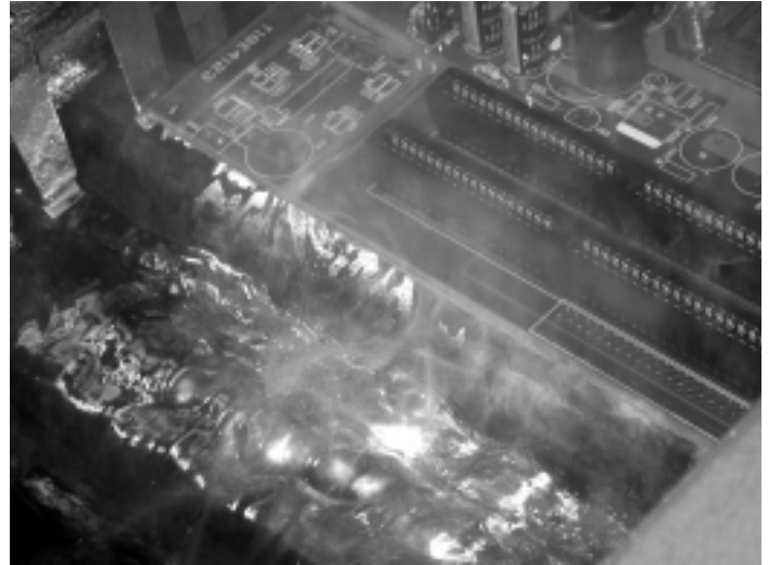
PCB passing over solder wave.
