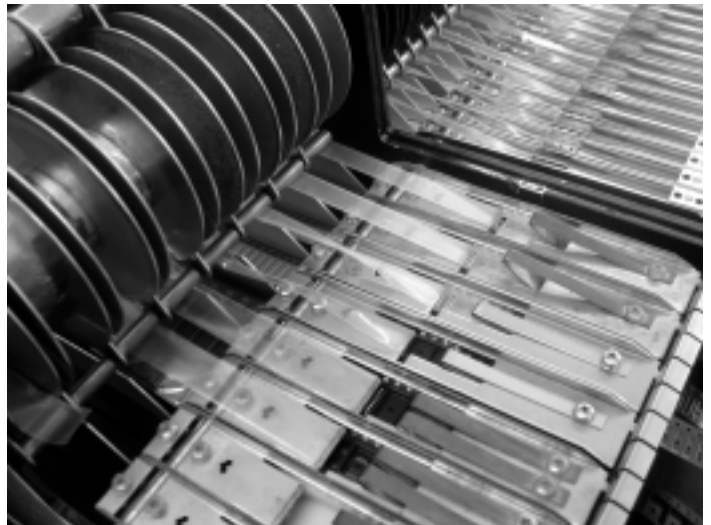
This is a close-up of the component-intake mechanism of one of our pick & place machines. A twelve-inch leader is necessary to wind the tape on the uptake spool.
